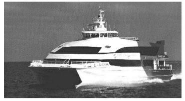
Type: Austal/Nautica 42 passenger catamaran Built: 1998/1999 Length: 42,16 meter. Beam: 13,5 meter Registered for Passengers: 358 Propulsion power: 2 x MTU, 16v 4000 M79, each of 2320 kW Speed: 35 knots
